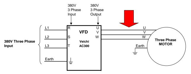
Input power to be connected to R, S & T . Input earth to be connected to earth Output power (marked "Motor") to be connected to motor U,V & W. VFD earth
