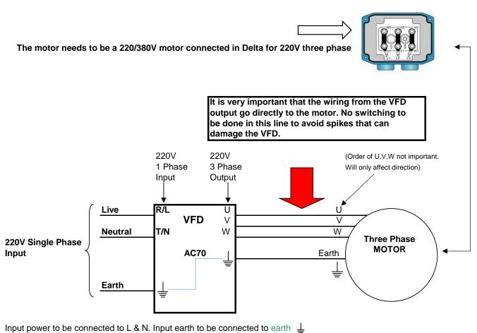
Motor to be connected to U,V & W and earth ↓
